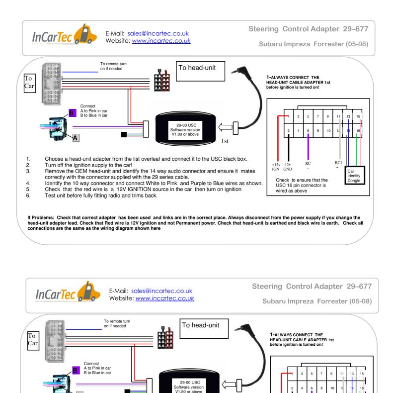
If Problems: Check that correct adapter has been used and links are in the correct place. Always disconnect from the power supply if you change the head-unit adapter lead. Check that Red wire is 12V ignition and not Permanent power. Check that head-unit is earthed and black wire is earth. Check all connections are the same as the wiring diagram shown here
